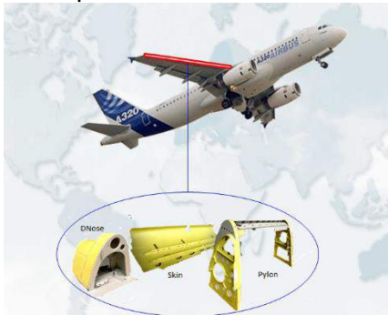
Figure 1 Illustration of Components Dnose, Pylon and Skin
