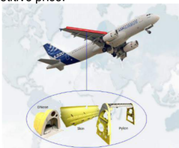
Figure 1 Illustration of Components Dnose, Pylon and Skin
