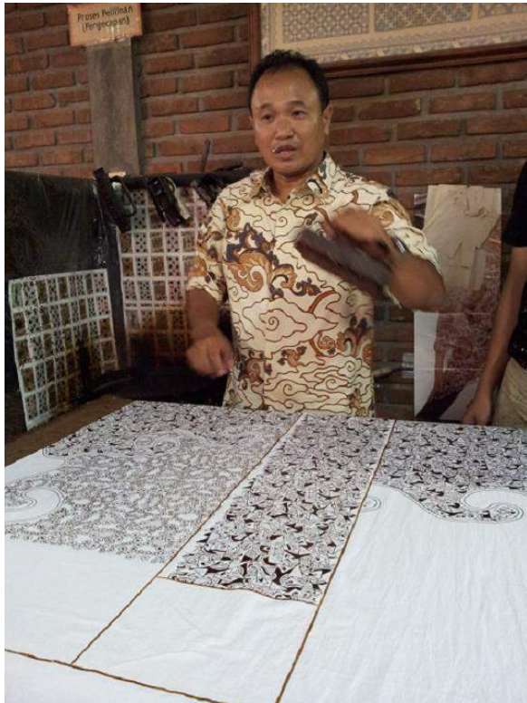
Figure 1. Stamping in Batik Cap
